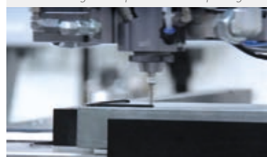
Robot for fitting bi-component form-in-place gasket
