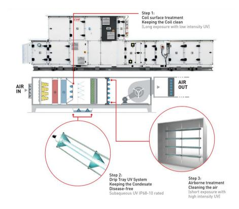
UV-C lamps installed at strategic points within the AHU enclosure flood vulnerable areas in high energy, cleansing UV-C light.
